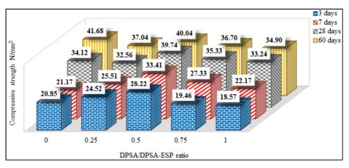
Figure 6. Variation of curing age on the mortar compressive strength at various DPSA/DPSA-ESP ratio for 4 wt. % cement replacement.
