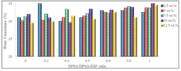
Figure 4. Variation of DPSA/DPSA-ESP ratio on the water consistence of cement blends at various cement replacements.
