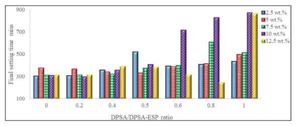
Figure 3. Variation of DPSA/DPSA-ESP ratio on the Final setting time of cement blends at various cement replacements.
