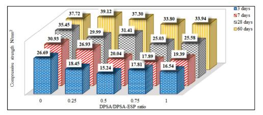
Figure 8. Variation of curing age on the mortar compressive strength at various DPSA/DPSA-ESP ratio for 8 wt. % cement replacement.
