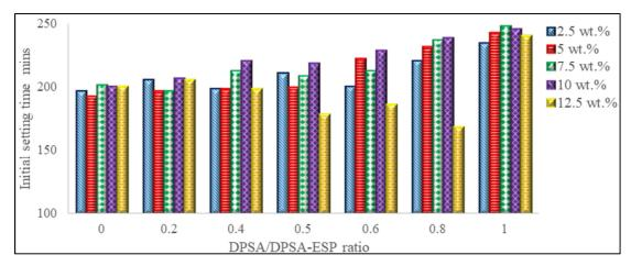
Figure 2. Variation of DPSA/DPSA-ESP ratio on the Initial setting time of cement blends at various cement replacements.
