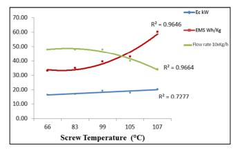
Figure 7. Flow rate, power and specific mechanical energy of the press as a function of the temperature.
