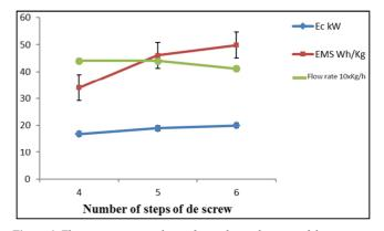
*Figure 6.* Flow rate, power and specific mechanical energy of the press as a function of the number of the steps of the screw.
